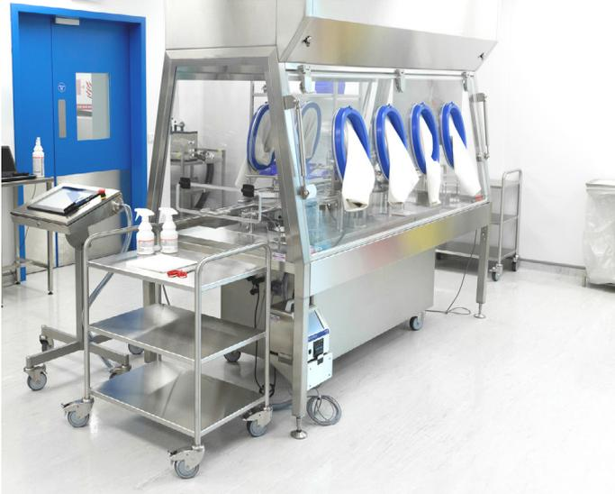
According to EU GMP Annex 1, an isolator is “An enclosure capable of being subject to reproducible interior bio-decontamination, with an internal work zone meeting Grade A conditions that provides uncompromised, continuous isolation of its interior from the external environment”. Isolators have several features to maintain Grade A conditions and isolation from the external environment such as:
