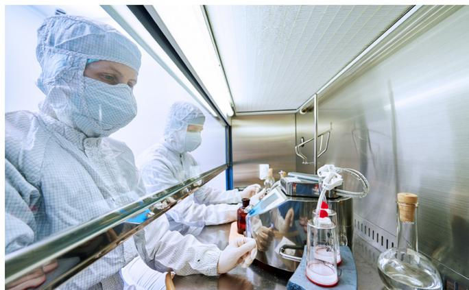
*Gowned operator performing sterility testing in a laminar air flow hood*
