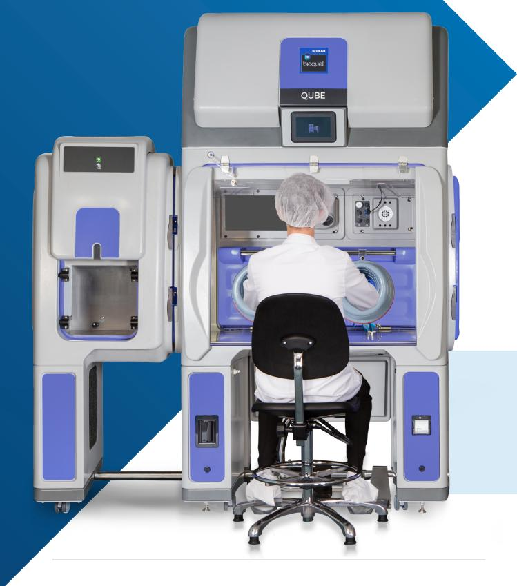
Ecolab's Bioquell Qube provides an aseptic ISO 5 / Grade A environment and includes integrated Bioquell Hydrogen Peroxide Vapour technology, achieving a validated 6-log sporicidal kill on every exposed surface within operating areas.
