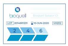
1 The Bioquell Isolator CI without any exposure to hydrogen peroxide vapor.
