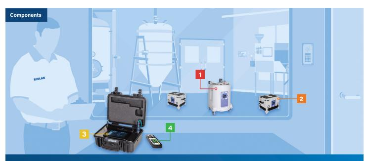
Vaporizers are placed strategically to emit the vapor and can be networked with multiple vaporizers to cover large volume areas.
