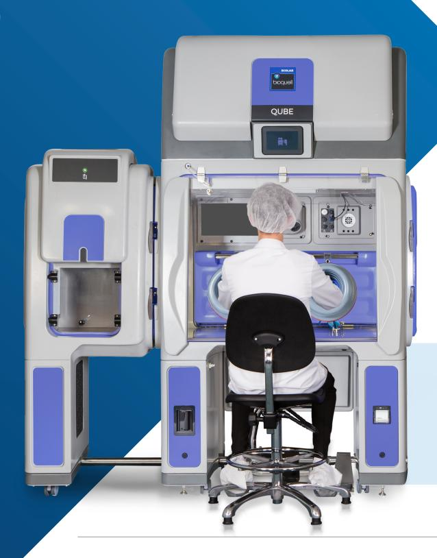
Ecolab's Bioquell Qube provides an aseptic ISO 5 / Grade A environment and includes integrated Bioquell Hydrogen Peroxide Vapor\* technology, achieving a validated 6-log sporicidal kill on exposed surfaces within operating areas.
